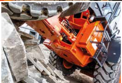
The optional belly guard provides added protection.
