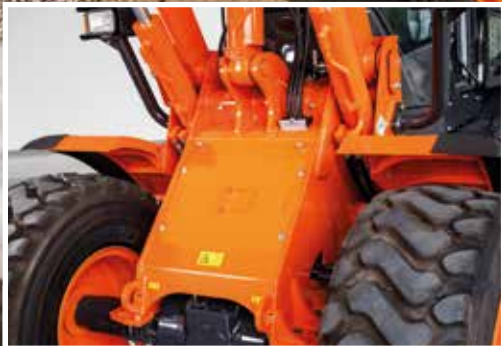
Reinforced front frame in the ZW140-6, 150-6 and 150PL-6.
