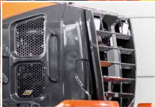
Wide fin coolers reduce heat and increase radiator durability
